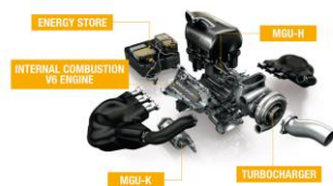
How ERS looks inside the Formula 1 engine 9
